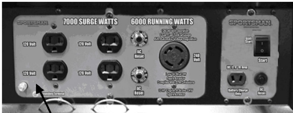
Figure 3 - Attaching the Grounding Wire to this Generator
