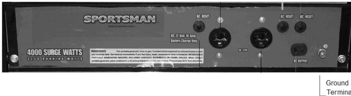
Figure 3 - Attaching the Grounding Wire to this Generator
