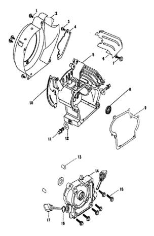
FIG.1 CRANKCASE UNIT (A152F01-00)
