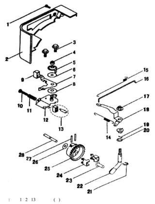
Note: The parts of No.1,2 and 13 only exist in the engine for the high-pressure pump
