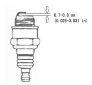
Figure 9 - Measuring the spark plug gap
