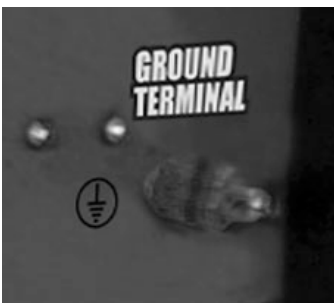
Figure 3 The Grounding Terminal is located on the front of the generator.
