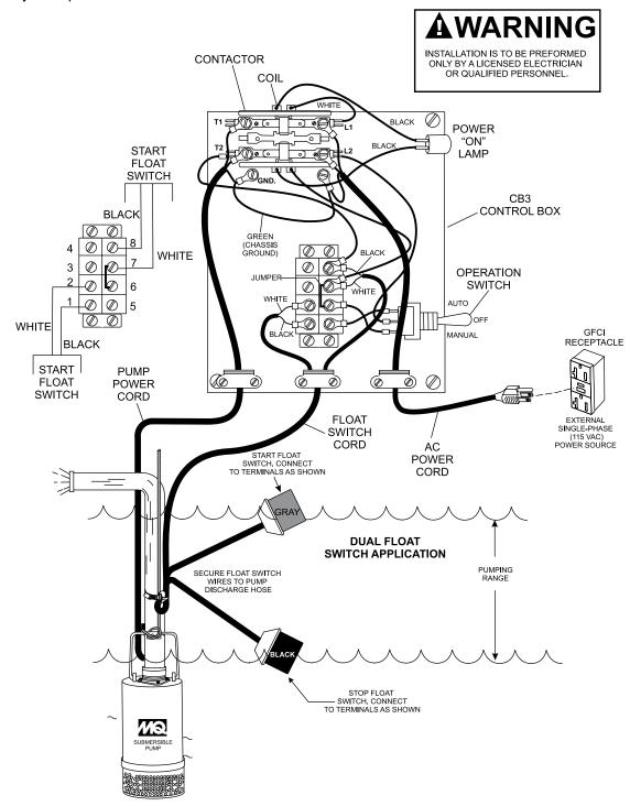
Figure 7. CB3 Control Box abd Dual Float Switch Application Diagram
