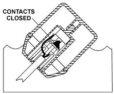
Figure 4. Float Switch (Closed)
