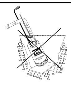
Figure 10. Submersible Pump Tilted (Incorrect Position)
