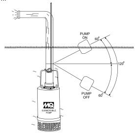
Figure 3. Pumping Range (Float Switch)
