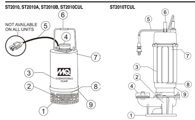
Figure 2. Submersible Pump Components
