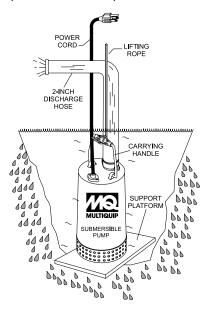
Figure 9. Submersible Pump Upright (Correct Position)
