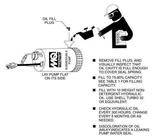
Figure 12. Checking Hydraulic Oil
