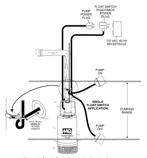
Figure 6. Single Float Switch Application Diagram
