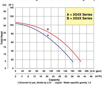
Performance of Engine Driven Solids Handling Pumps
