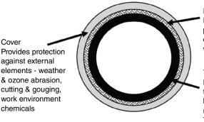
Reinforcement Provides strength to resist pressure and vacuum. Uses combinations of textile and wire
