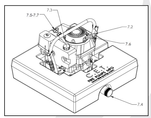
7.4. Connect the discharge hose. Make sure that there is a rubber seal on the adapter and screw it tight. Verify the water source to be used is clear of sand and/or small rocks, if you have any doubt about your water source, we recommend you use a strainer. If sand enters your pump it would damage the seal and wear rings, reducing useful life. The water source should be at least 12" deep.
