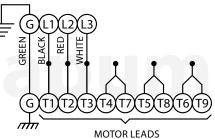
Figure 5CableMotor Lead NumberGreenGreenBlack1Red2White34 and 7 together5 and 8 together6 and 9 together
