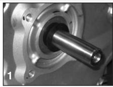
3. To install the carbon seal half into the rear bracket use a tool such as a 1 ½" pipe nipple or arbor press to give even pressure on the metal flange of the seal housing during installation. Gently press the seal into position until it bottoms.
