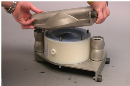
Remove side housing [1] and suction/discharge ports [2].
