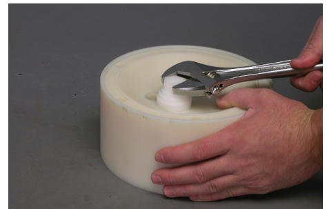
To remove the air control system, screw off both end caps using the plastic mounting tool delivered with the pump. Take out main and pilot piston.
