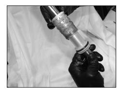
STEP 4 Remove "O-rings" and "inner spacer".
