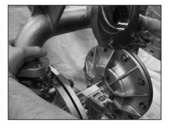
STEP 5 Remove the "Suction Manifold".
