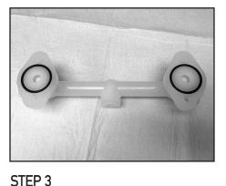
Remove the "O-Ring", "Valve Seat" and "Ball" from the "Discharge Manifold".
