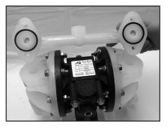
STEP 2 Remove the "Discharge Manifold".
