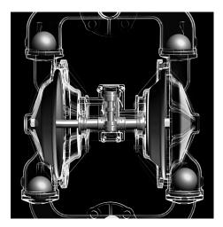
The air-valve directs pressurized air behind the left diaphragm, causing the left diaphragm to move outward (to the left).
