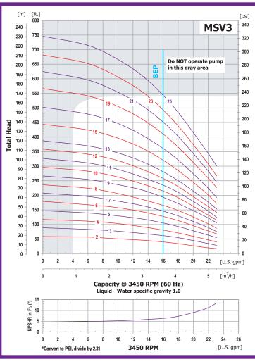
Maximum Working Pressure 232 PSI [1600 kPa] Maximum Temp 180° F
