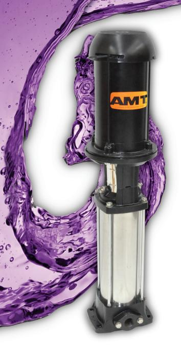
These AMT commercial/industrial centrifugal pumps are non-self-priming (gravity feed) units designed to handle high-pressure low flow liquid transfer applications where no suction lift is required. Typical installations include: hot and chilled water, boiler feed, condensate return, irrigation, high pressure washdown, booster service, and fire protection/sprinkler systems—often referred to as a Jockey Pump. These pumps have NOT been investigated for use in potable (drinking) water systems.
