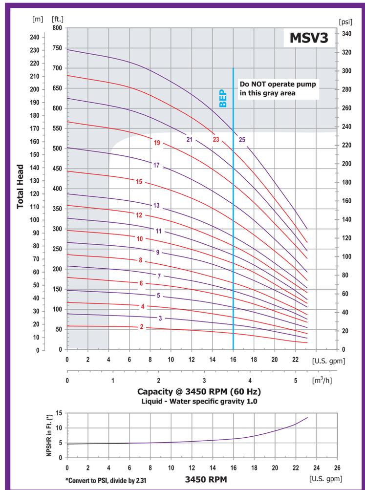
Maximum Working Pressure 232 PSI [1600 kPa]      Maximum Temp 180° F
