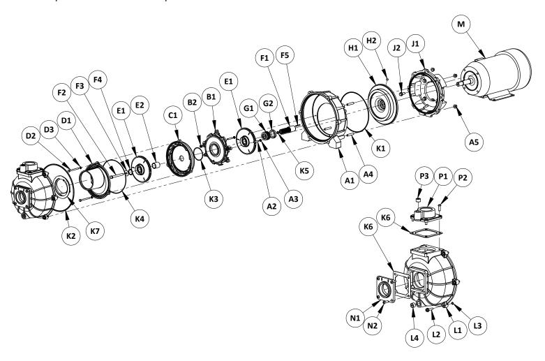
Figure 1 - Repair Parts Illustrations
